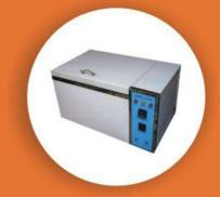
Accelerated Curing Tank having capacity to accommodate Concrete Cubes of 150mm size with a facility for accelerated curing by Boiling water method up to temperature range: 100 +/- 2 deg.C . Also it will have capacity for curing by warm water method at temperature 55 +/- 2 deg.C.
